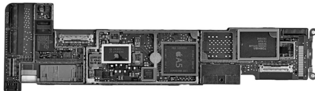
FIGURE 1.8 The logic board of Apple iPad 2 in Figure 1.7 . The photo highlights five integrated circuits. The large integrated circuit in the middle is the Apple A5 chip, which contains dual ARM processor cores that run at 1 GHz as well as 512 MB of main memory inside the package. Figure 1.9 shows a photograph of the processor chip inside the A5 package. The similar-sized chip to the left is the 32 GB flash memory chip for non-volatile storage. There is an empty space between the two chips where a second flash chip can be installed to double storage capacity of the iPad. The chips to the right of the A5 include power controller and I/O controller chips. (Courtesy iFixit, www.ifixit.com )
