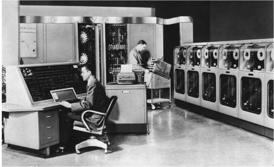
FIGURE e1.12.2 UNIVAC I, the first commercial computer in the United States. It correctly predicted the outcome of the 1952 presidential election, but its initial forecast was withheld from broadcast because experts doubted the use of such early results.
