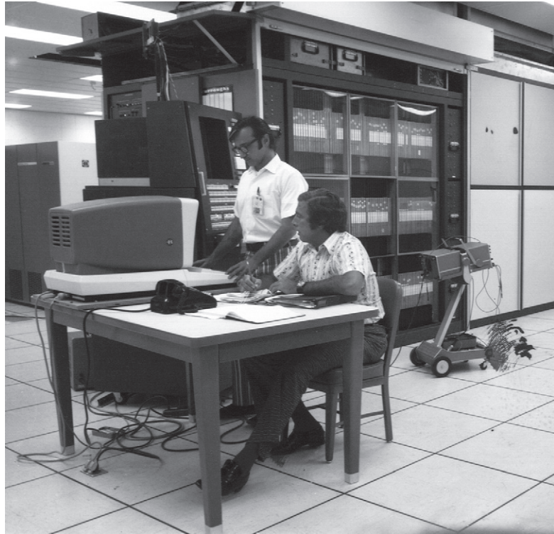
FIGURE e6.15.1 The Illiac IV control unit followed by its 64 processing elements. It was perhaps the most infamous of supercomputers. The project started in 1965 and ran its first real application in 1976. The 64 processors used a 13-MHz clock, and their combined main memory size was 1 MB: 64 \times 16 KB. The Illiac IV was the first machine to teach us that software for parallel machines dominates hardware issues. Photo courtesy of NASA Ames Research Center.
