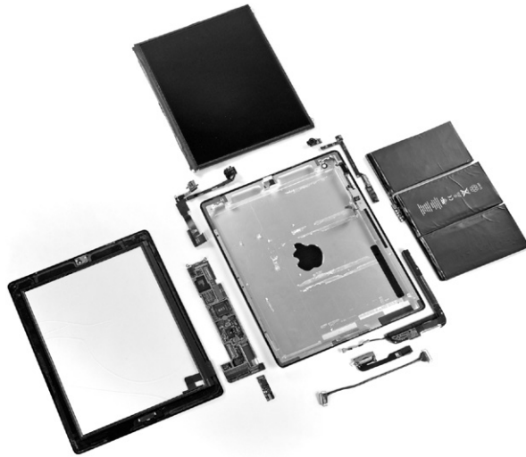
FIGURE 1.7 Components of the Apple iPad 2 A1395. The metal back of the iPad (with the reversed Apple logo in the middle) is in the center. At the top is the capacitive multitouch screen and LCD. To the far right is the 3.8V, 25 watt-hour, polymer battery, which consists of three Li-ion cell cases and offers 10 hours of battery life. To the far left is the metal frame that attaches the LCD to the back of the iPad. The small components surrounding the metal back in the center are what we think of as the computer; they are often L-shaped to fit compactly inside the case next to the battery. Figure 1.8 shows a close-up of the L-shaped board to the lower left of the metal case, which is the logic printed circuit board that contains the processor and the memory. The tiny rectangle below the logic board contains a chip that provides wireless communication: Wi-Fi, Bluetooth, and FM tuner. It fits into a small slot in the lower left corner of the logic board. Near the upper left corner of the case is another L-shaped component, which is a front-facing camera assembly that includes the camera, headphone jack, and microphone. Near the right upper corner of the case is the board containing the volume control and silent/screen rotation lock button along with a gyroscope and accelerometer. These last two chips combine to allow the iPad to recognize six-axis motion. The tiny rectangle next to it is the rear-facing camera. Near the bottom right of the case is the L-shaped speaker assembly. The cable at the bottom is the connector between the logic board and the camera/volume control board. The board between the cable and the speaker assembly is the controller for the capacitive touchscreen. (Courtesy iFixit, www.ifixit.com )
