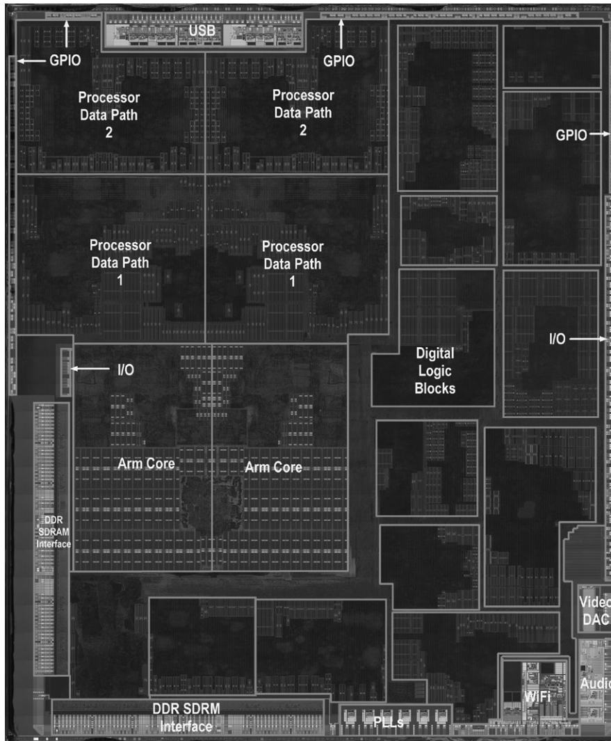
FIGURE 1.9 The processor integrated circuit inside the A5 package. The size of chip is 12.1 by 10.1 mm, and it was manufactured originally in a 45-nm process (see Section 1.5). It has two identical ARM processors or cores in the middle left of the chip and a PowerVR graphics processing unit (GPU) with four datapaths in the upper left quadrant. To the left and bottom side of the ARM cores are interfaces to main memory (DRAM). (Courtesy Chipworks, www.chipworks.com )
